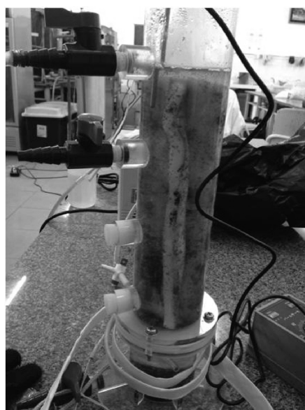
Figure 7. Attached biomass observation after 193 days
