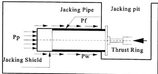
Figure 3. Components of the Jacking Force during the construction phase [7]
