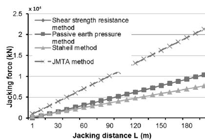
b) Comparison diagram in the lubricated case
