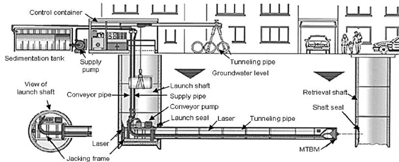
**Figure 1. Schematic of Microtunneling Operation [1]**
