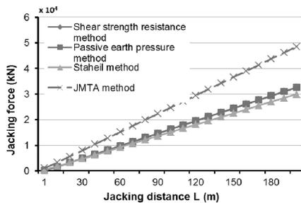
a) Comparison diagram in the unlubricated case
