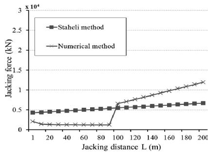
b) Using lubricate ( $\mu = 0.1$ )
