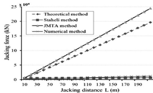
Figure 7. Comparison diagram when using lubricate ( $\mu = 0.1$ )
