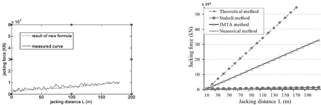
a) Numerical method vs. Measured data [16]
