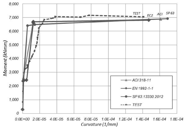
Figure 11. Experimental and theoretical moment-curvature diagrams of D1.1-2φ8
