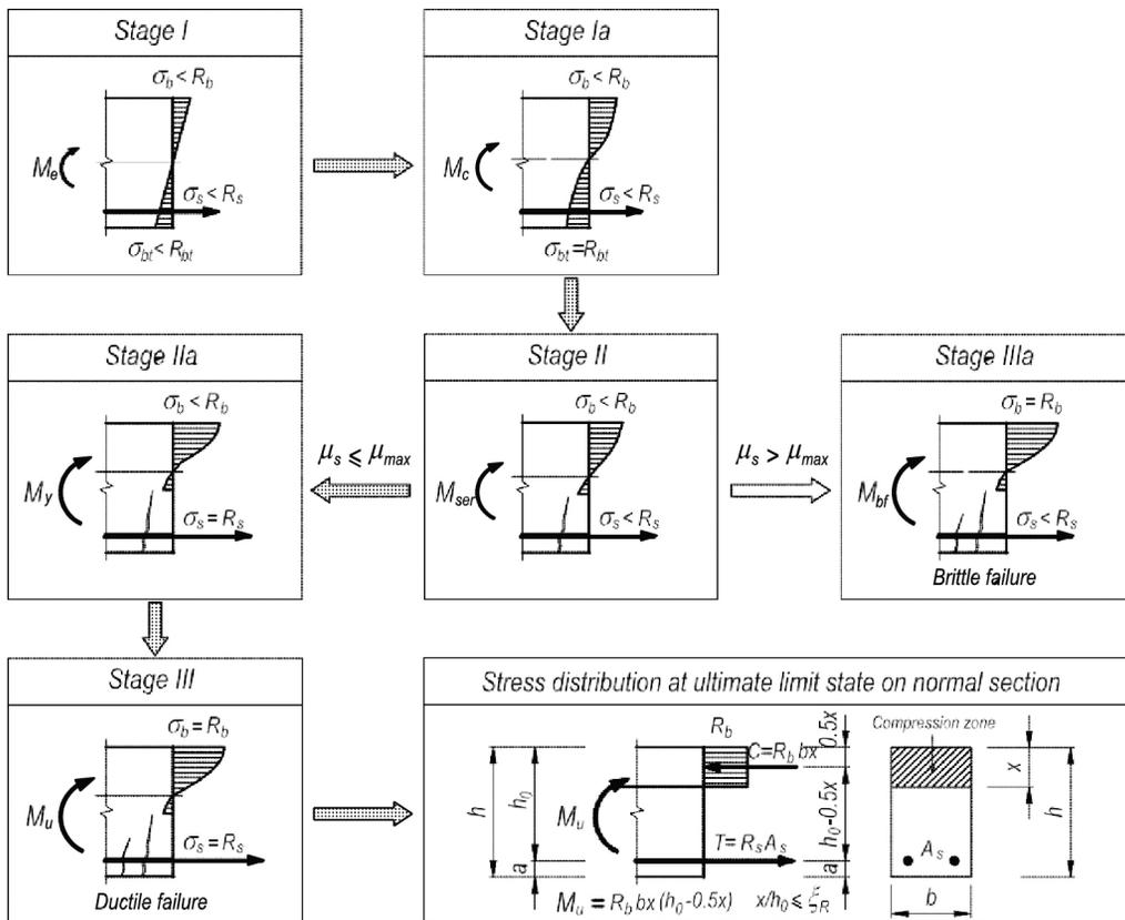
**Figure 2. Flexural behavior and strength calculation of RC beams to TCVN 5574:2012**
