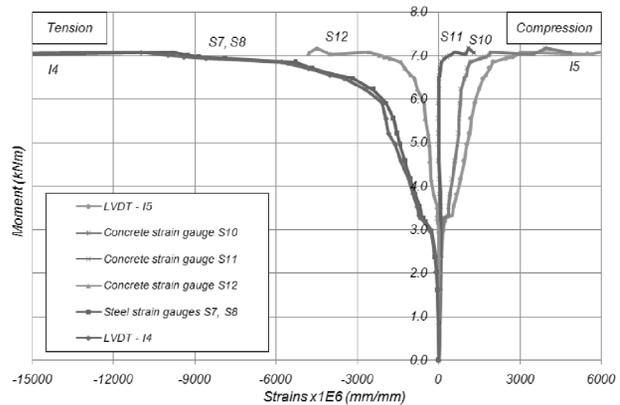
**Figure 9. The development of strain along the normal section of D1.1-2φ8**
