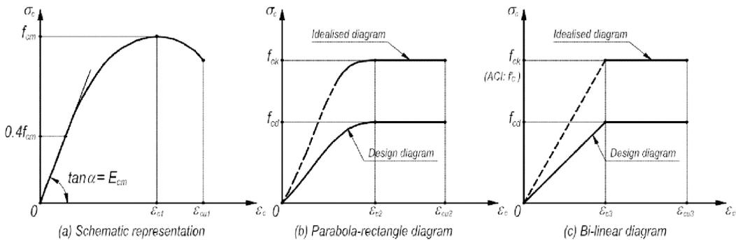
**Figure 3. Compressive stress-strain relationship of concrete specified in EC2**
