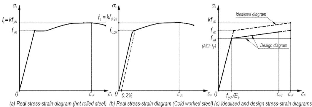
**Figure 4. Stress-strain relationship of reinforcing steel specified in EC2**
