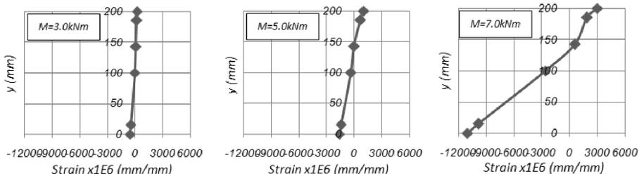
**Figure 10. The distribution of strain along the normal section of D1.1-2φ8**
