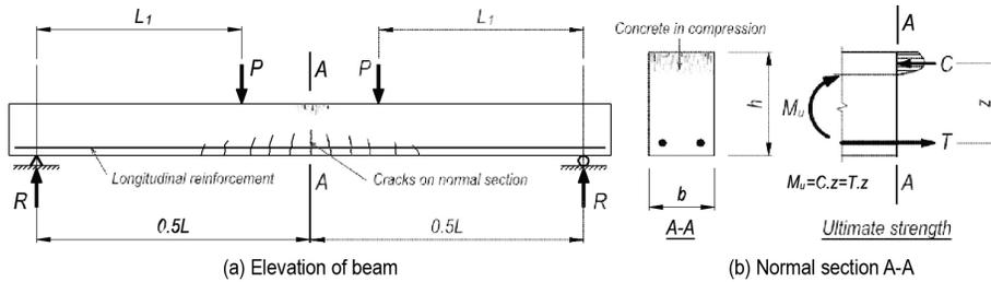
**Figure 1. RC beam subjected to bending moment**
