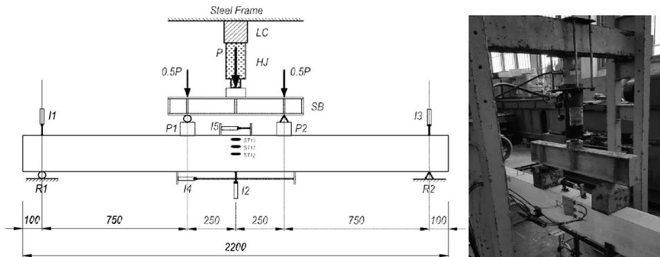
**Figure 8. Test set-up**
