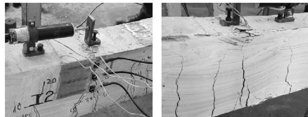
Figure 13. Failure at mid-span
