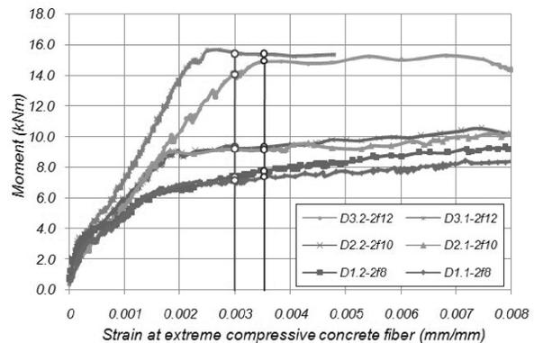
Figure 14. Experimental relationship between moment and extreme concrete compressive strain
