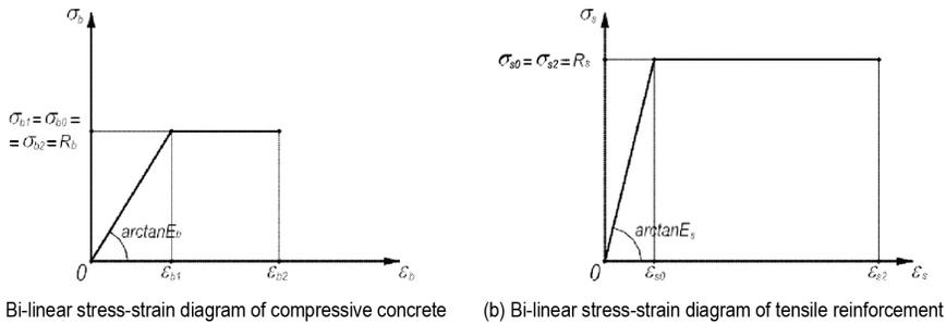
Figure 6. Simplified stress-strain relationship of material specified in SP 63.13330.2012
