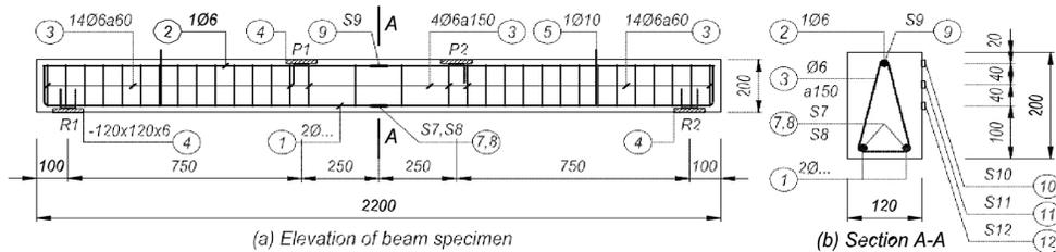
Figure 7. Details of beam specimens
