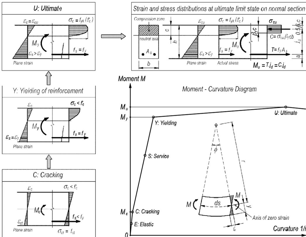
Figure 5. Flexural behavior and strength calculation of RC beams to ACI 318-11 and EC2
