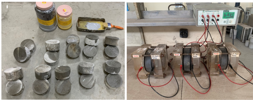
Figure 12. Chloride-ion penetration test setup
