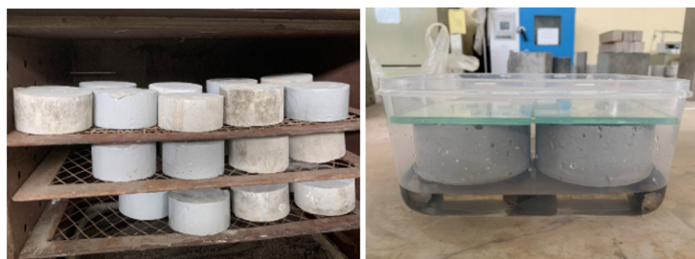
Figure 9. Capillary water absorption coefficient test setup
