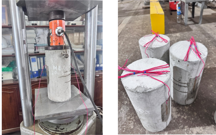
Figure 3. Experimental setup for uniaxial compression tests and strain measurement of cylindrical EPS concrete specimens according to RILEM CPC 19
