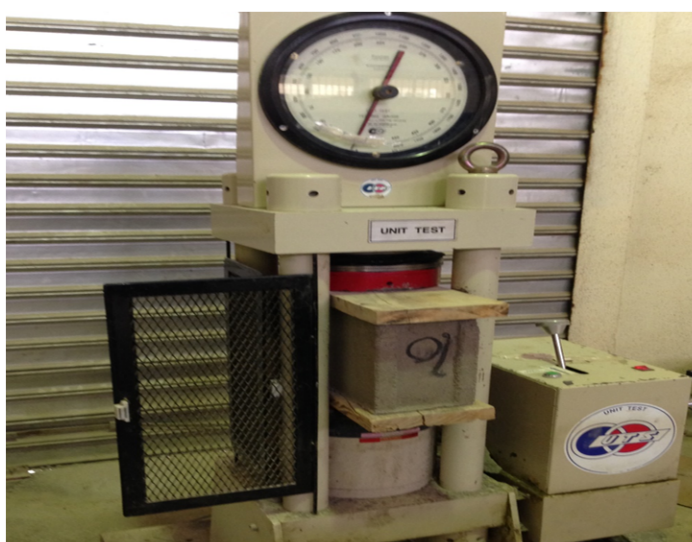
Figure 2. Compression testing machine with seashell block
