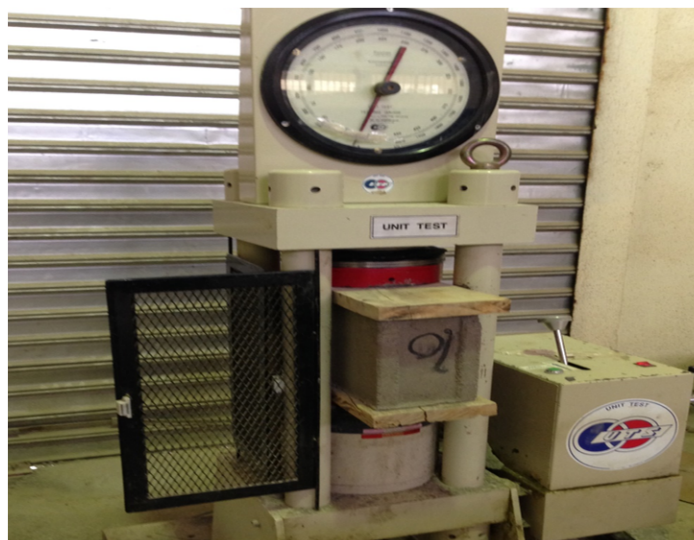
Figure 2. Compression testing machine with seashell block
