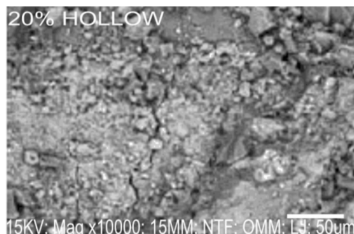
Figure 6. SEM for 20% seashell percentage replacement of natural fine aggregates
