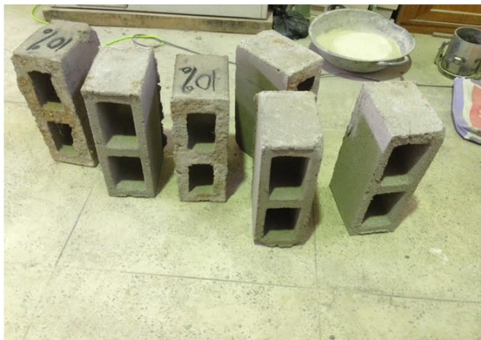
Figure 1. Batched Hardened Hollow block samples with Senilia senilis shells
