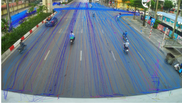
Figure 4. Vehicle trajectory H20 reference point at the Nguyen Trai – Nguyen Van Loc intersection
