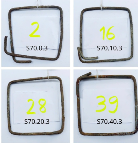
Figure 7. Surface of lateral reinforcing steel specimens after testing – Group 2 (3V)
