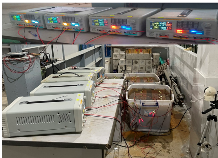
Figure 3. Inducing corrosion of lateral reinforcement in RC columns
