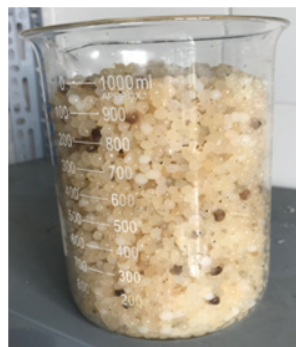
(b) PVA/ \text{NaNO}_3 granules after 5 weeks in SBR operation
