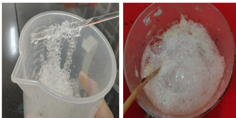
Figure 3. Foam observed due to PVA/ \text{H}_3\text{BO}_3 granules breakage after aeration test
