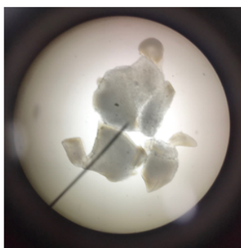
(c) PVA/ \text{NaNO}_3 granules with attached microorganism in microscopy \times 20
