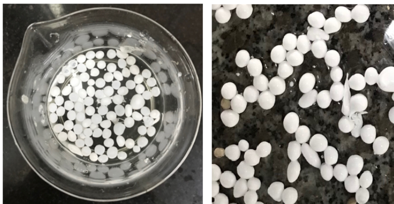
Figure 4. Digital camera images of strong PVA/NaNO 3 granules after aeration test
