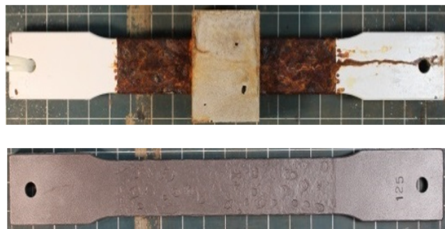
Figure 3. Corroded specimens after cleaning
