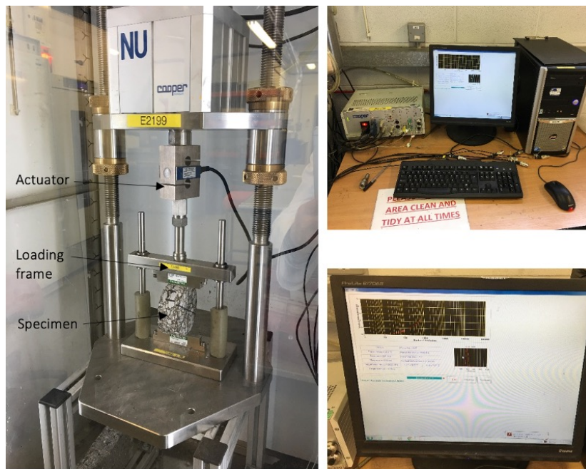
Figure 5. Schematic of ITFT at NTEC
