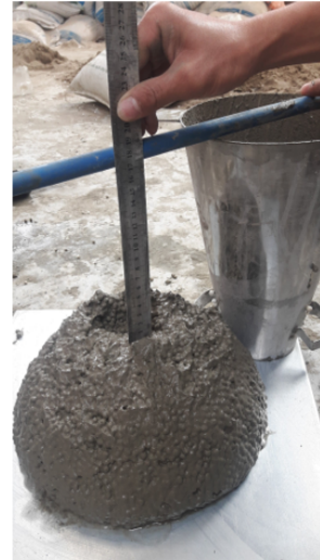
Figure 4. Determining the slump of the concrete mixture
