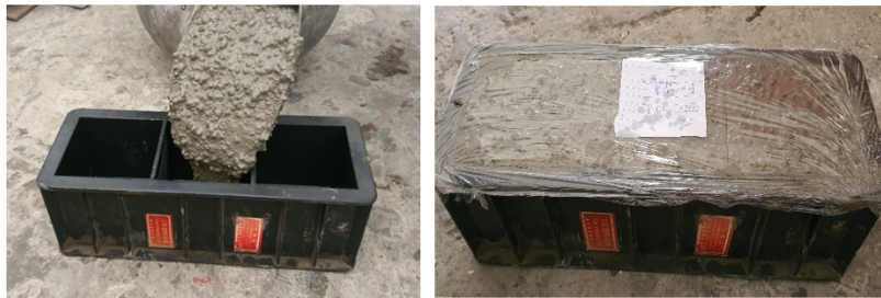
Figure 2. Casting and curing the EPS-C
