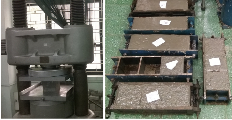
Figure 1. Preparation of concrete samples and compressive strength testing
