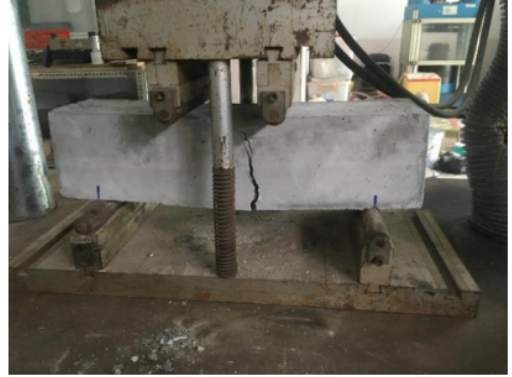
(b) Formation and slow extension of cracks from the tension area
