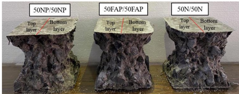
Figure 14. The visual inspection of the fractured surface of FGC samples after compression test
