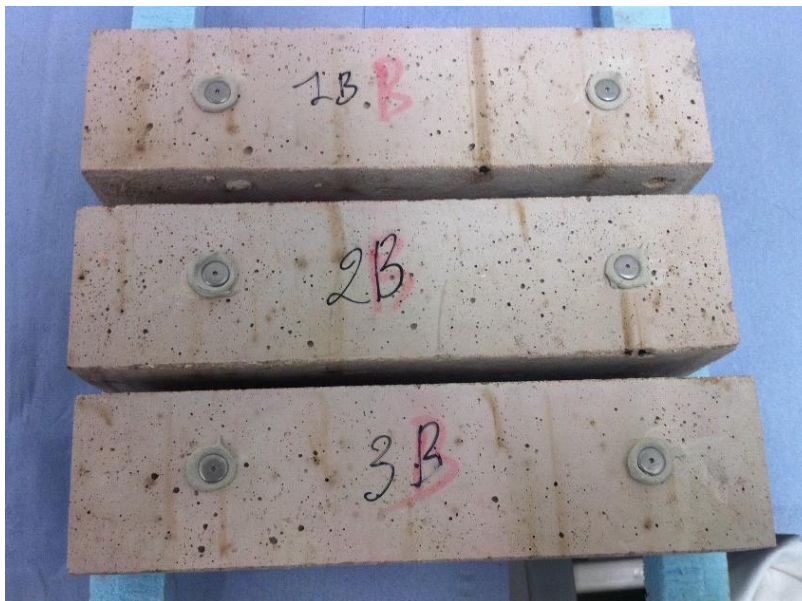
Figure 1. Shrinkage measurement of mortar samples
