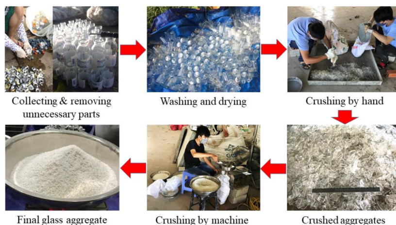
Figure 3. Procedures for the preparation of RGA
