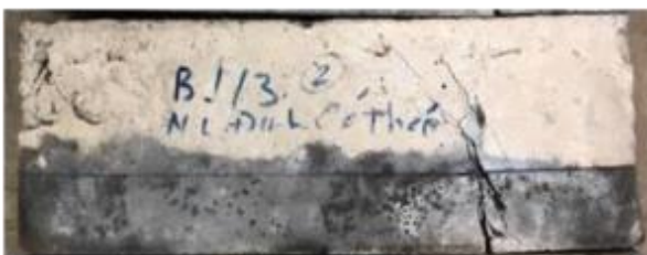
(g) Short 4 with one-third using HPFRC at bottom
