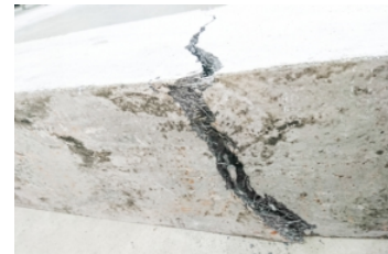
(h) Long 4 with one-third using HPFRC at bottom
