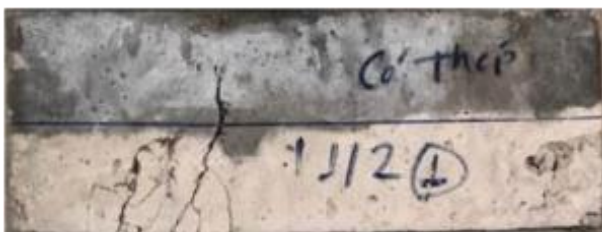
(i) Short 5 with one-half using HPFRC at top
