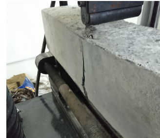
(b) Long 1 with full of HPFRC and no reinforcing bar
