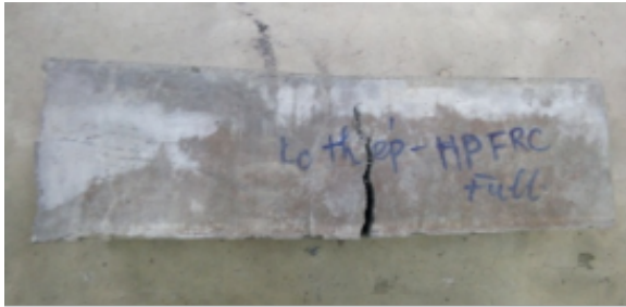
(a) Short 1 with full of HPFRC and no reinforcing bar
