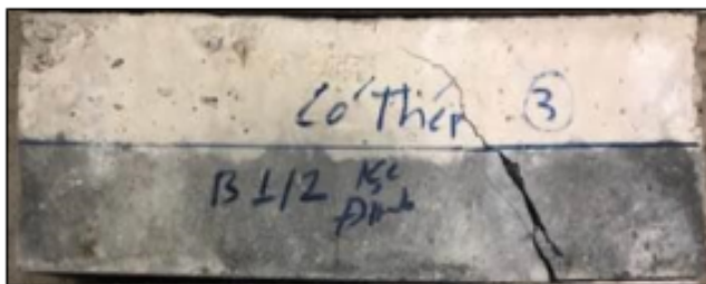
(e) Short 3 with one-half using HPFRC at bottom
