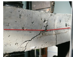
(j) Long 5 with one-half using HPFRC at top
