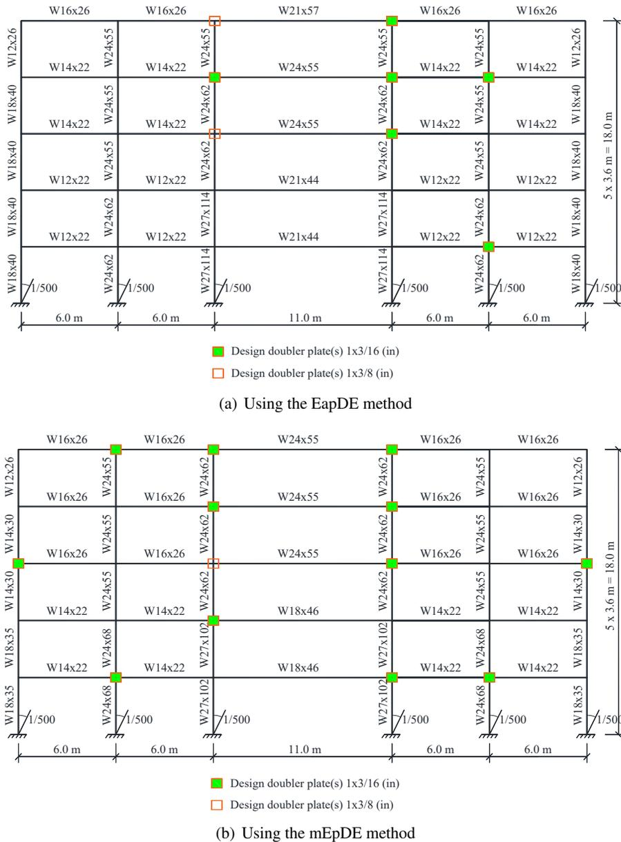
Figure 4. Best optimum design of five bay-five story steel frame
