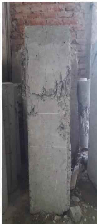
(b) Concrete spalling
