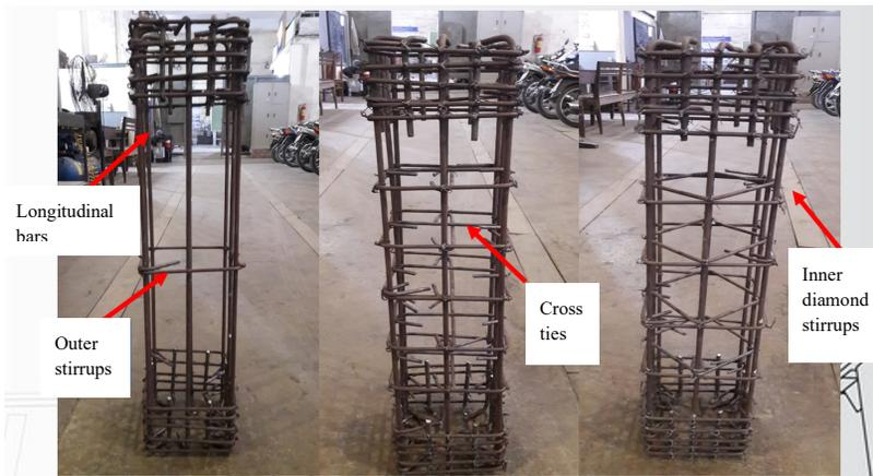
Figure 2. A photo of reinforcement cages of test specimens
