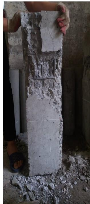
(c) Buckling of longitudinal bars and concrete crushing
