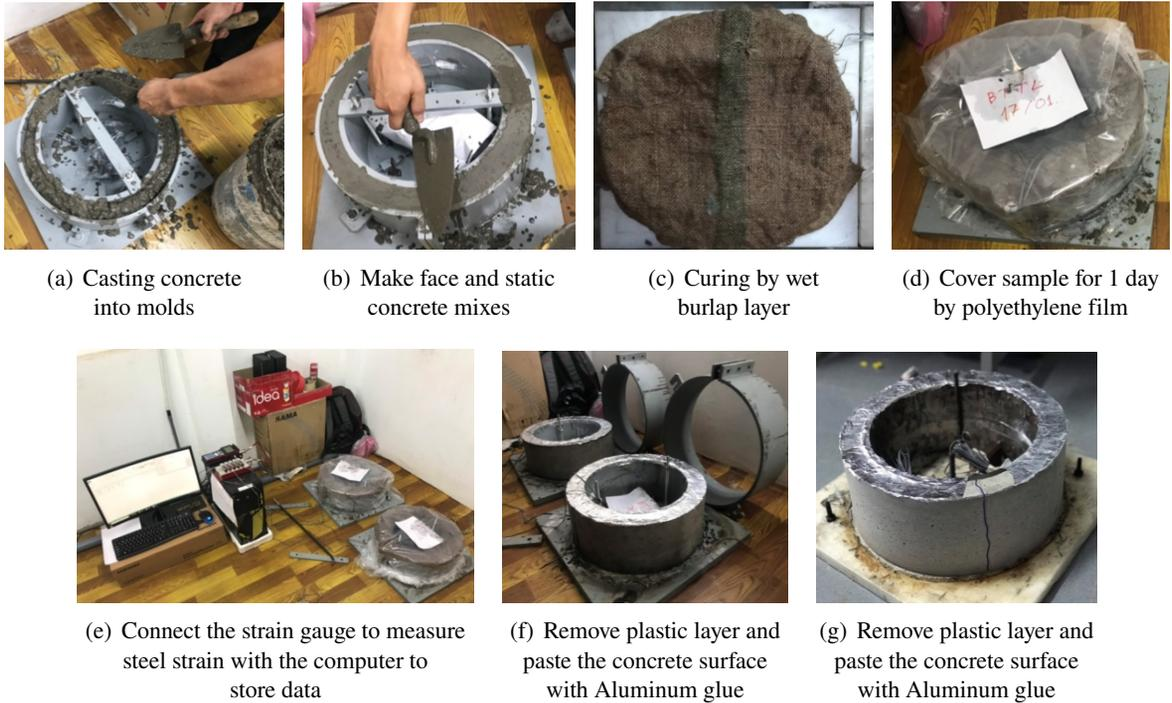
Figure 3. The experimental process of restrained ring test
