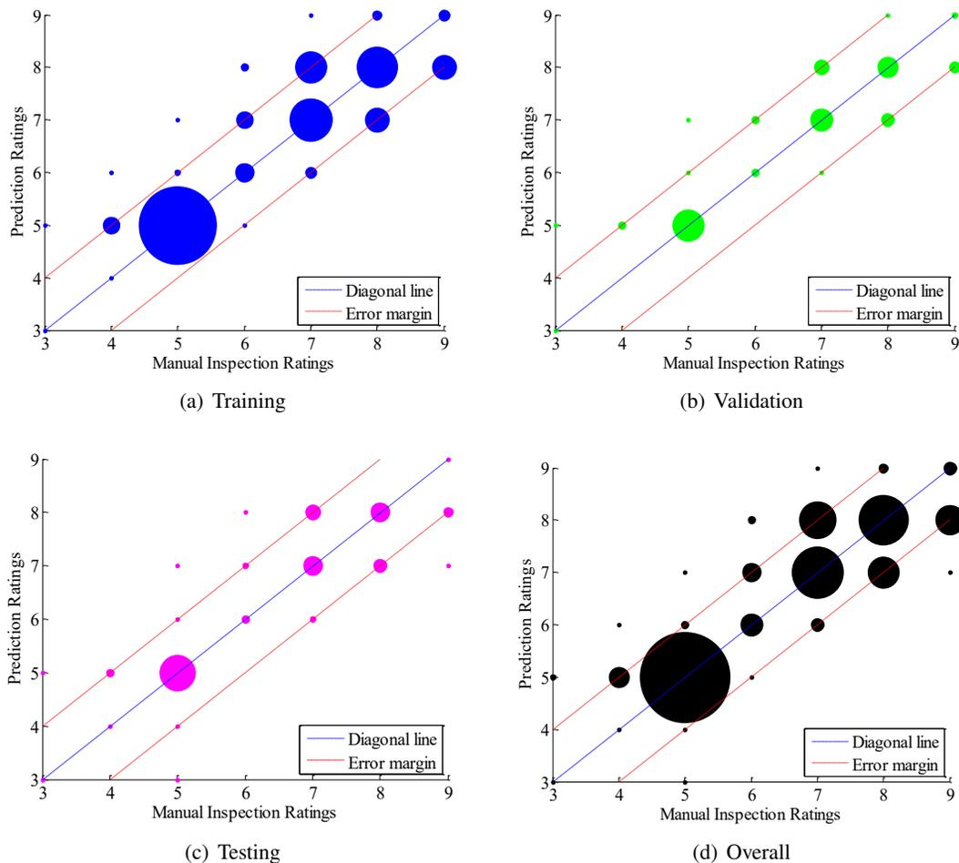
Figure 4. Bridge deck ratings – Bubble plots
