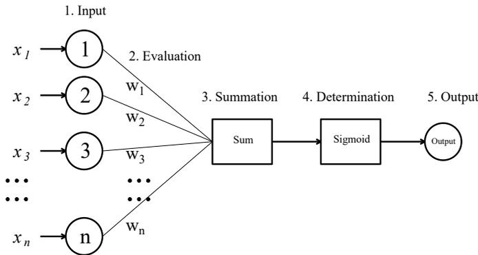
Figure 1. Components of a simple neuron
