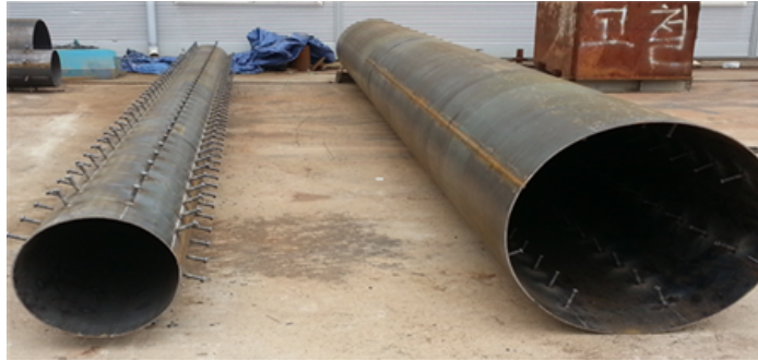
Figure 2. Detail of the steel tubes and shear connector system
