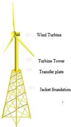
Figure 10. 3D model of Jacket support-structure wind turbine
