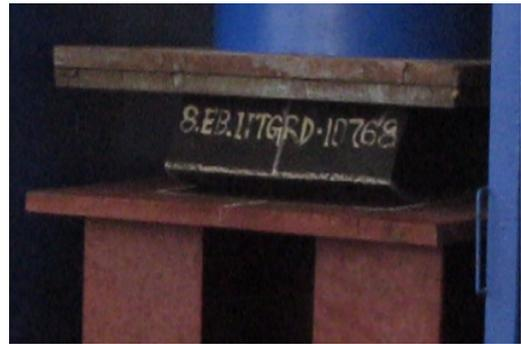
Figure 4. Deformed shape of U-FREI specimen at applied horizontal displacement of 80 mm
