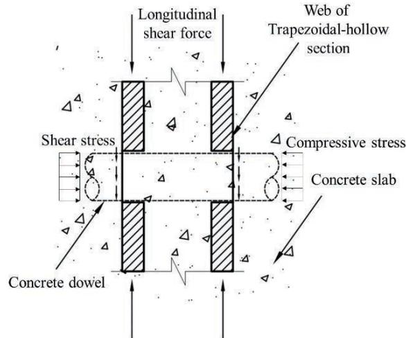
Figure 6. Stress state of concrete dowel
