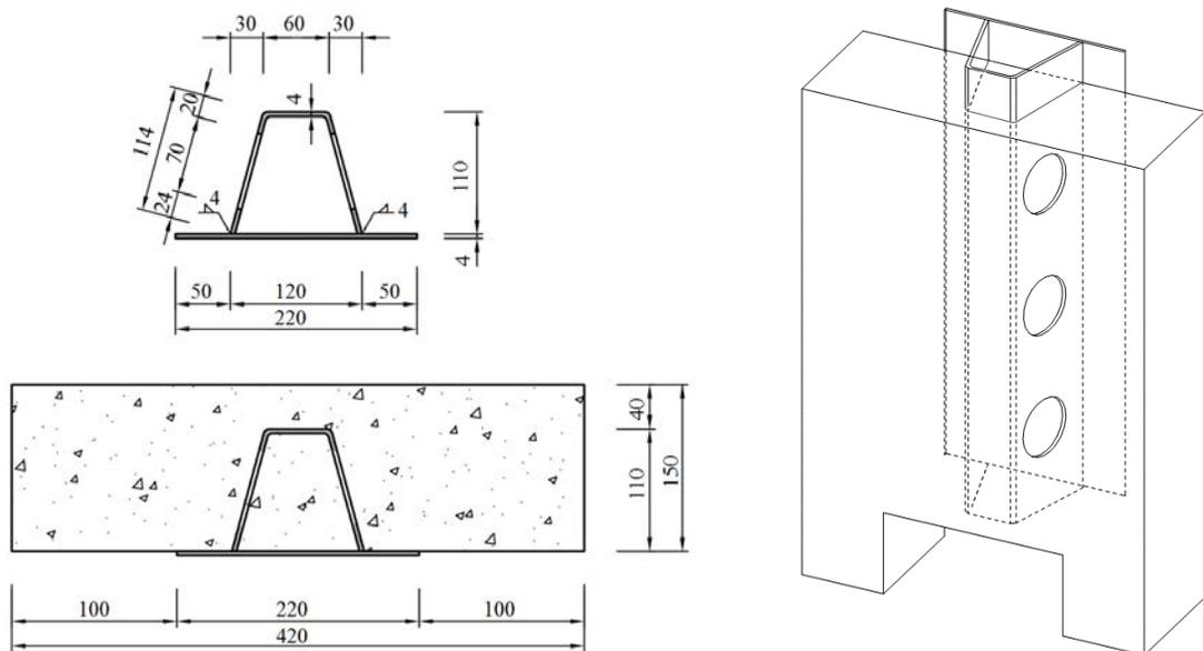
Figure 2. Dimensions and shape of push-out test specimens
