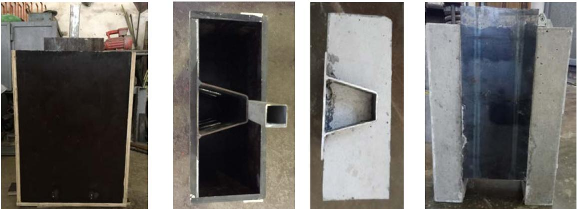
Figure 3. Formwork and finishing of the specimens
