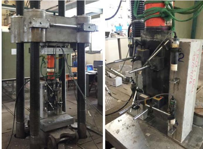
Figure 4. Push-out test set up
