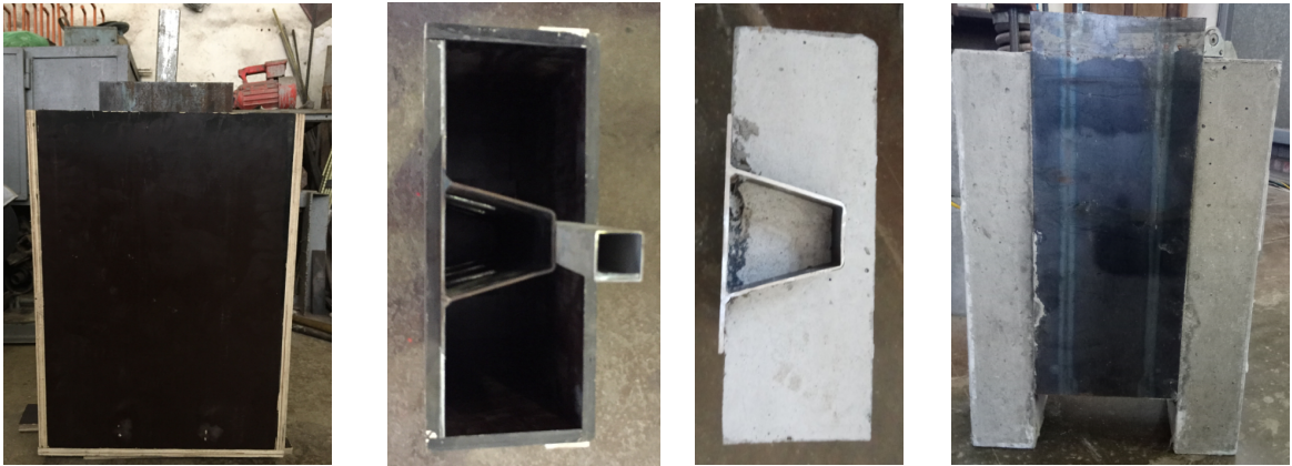
Figure 3. Formwork and finishing of the specimens
