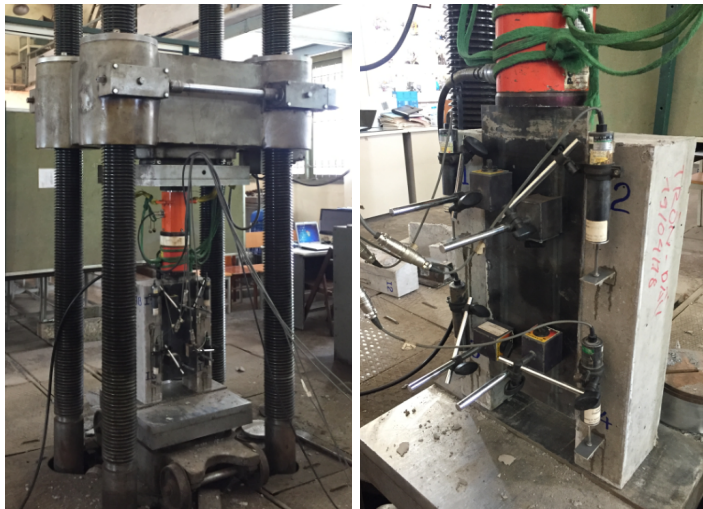
Figure 4. Push-out test set up
