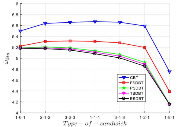
Figure 3. Effect of the face-core-face thickness ratio on non-dimensional fundamental natural frequency  $\bar{\omega}$  of FG sandwich beams
