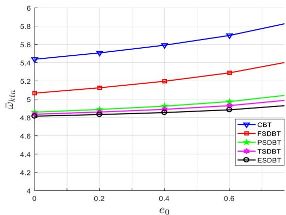
Figure 5. Effect of porosity coefficient of the porous core  $e_0$  on non-dimensional natural frequency  $\bar{\omega}$  of FG sandwich beams
