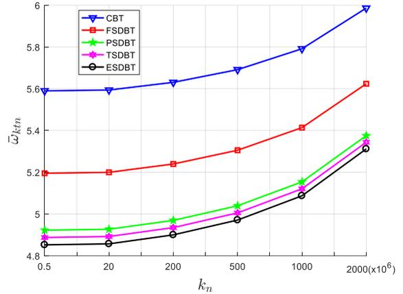
Figure 6. Effect of stiffness of Winkler elastic foundation  $k_n$  on non-dimensional natural frequency  $\bar{\omega}$  of sandwich beams
