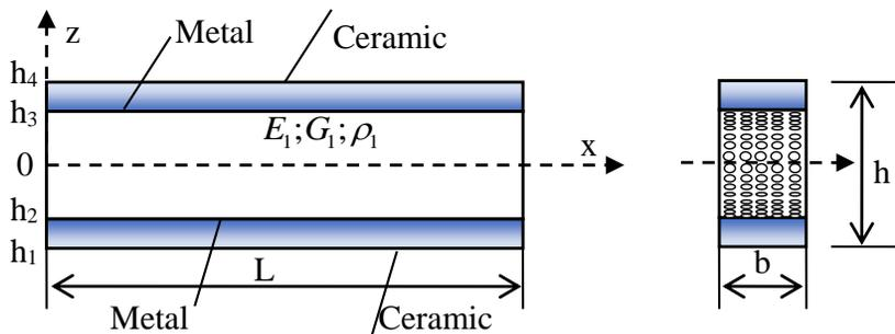
Figure 1. Sandwich beam with functionally graded porous core and FGM face layers
