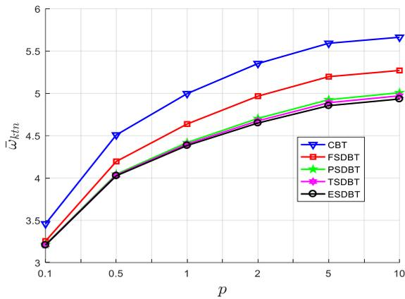
Figure 4. Effect of volume fraction index  $p$  of the face layers on non-dimensional fundamental natural frequency  $\bar{\omega}$  of FG sandwich beams
