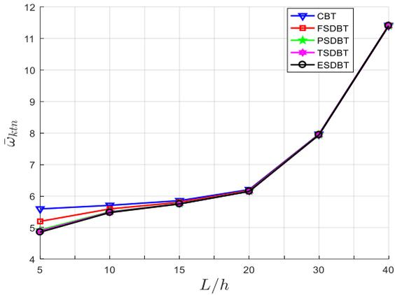
Figure 2. Effect of  $L/h$  ratio on non-dimensional natural frequency  $\bar{\omega}$  of 1-2-1 sandwich beam
